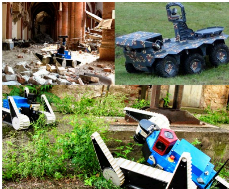
Urban Search & Rescue robots deployed to earthquake-hit area of Mirandola, Italy, 2012 as part of EU FP-7 project NIFTi and TRADR (top-left, bottom); Multipurpose UGV platform TAROS (top-right).
